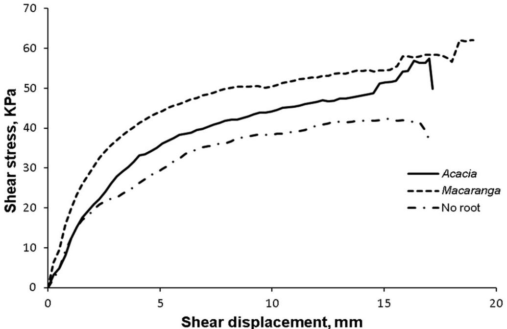
**Fig. 4. Relationship between shear stress and shear displacement of rooted and non-rooted soil samples (applying normal stress of 44.98 KPa).**
