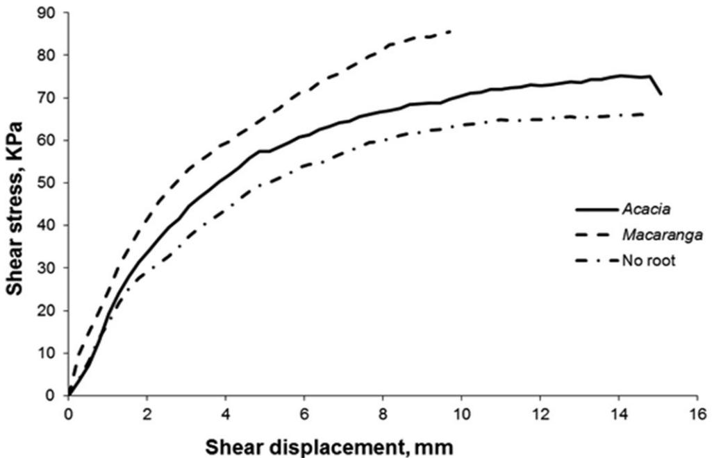
Fig. 6. Relationship between shear stress and shear displacement of rooted and non-rooted soil samples (applying normal stress of 138.19 KPa).
