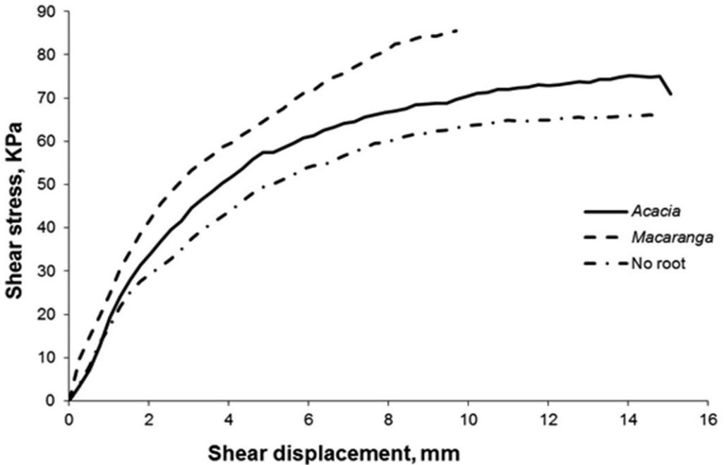
**Fig. 5. Relationship between shear stress and shear displacement of rooted and non-rooted soil samples (applying normal stress of 76.05 KPa).**
