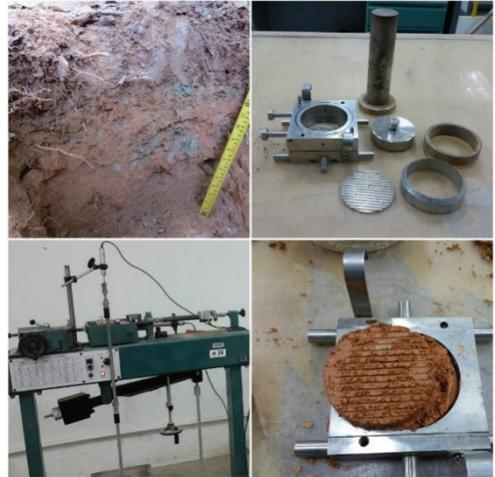
Fig. 2. The process of undisturbed soil sampling and analyzing with direct shear box machine.
