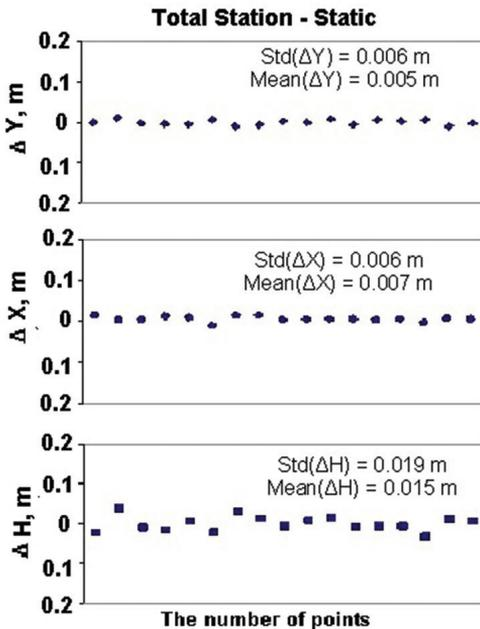
Fig. 6. Comparison of the coordinates of the 17 points in the project area between total station and static GPS surveys.
