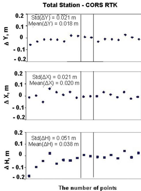
**Fig. 5. Comparison of the coordinates of the 17 points in the project area between total station and CORS RTK surveys.**
